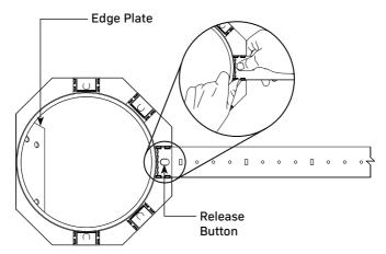
The in-ceiling speakers include an edge plate to secure if mounting the speaker against a joist.
