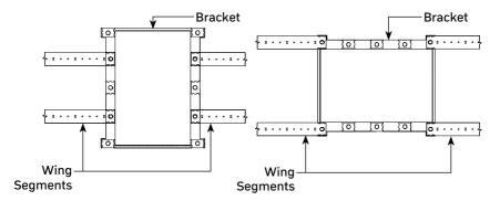
3. Use the 1" markers as a placement guide for aligning the brackets. Drive a screw through the metal wings to secure into the desired position.
