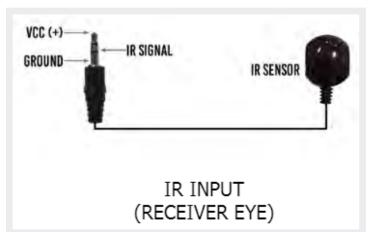
IR Direct Input from Control System (Transmitter Only) (Mono Tip to Tip/ Sleeve to Sleeve) (Dipswitch 5 = 1)
