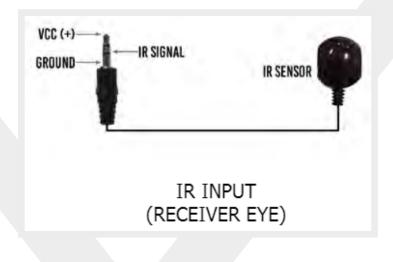
IR Direct Input from Control System (Transmitter Only) (Mono Tip to Tip/ Sleeve to Sleeve) (Dipswitch 5 = 1)
