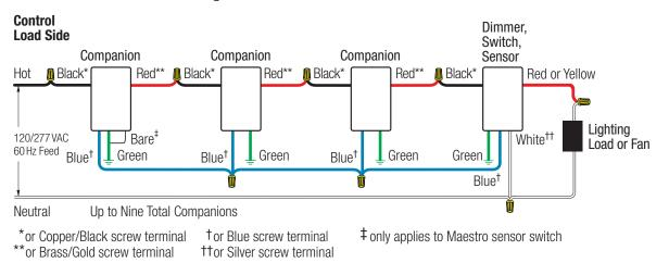
Load side 3-way wiring of multi-location control with neutral wire connection with mechanical switch
