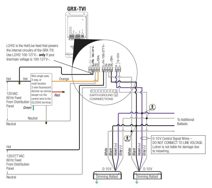
Some 0-10 V LED and fluorescent loads require low-end trim adjustments. Select a 3-wire dimmer that has an adjustable low-end trim. 0-10 VDC sink control
