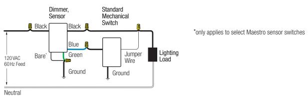
Single-pole wiring of multi-location control with neutral wire connection
