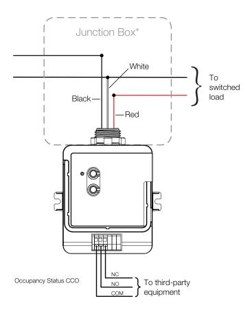
\*Some applications require the Vive PowPak module to be installed inside an additional junction box. For more information consult Lutron Application Note #423, Installing a PowPak Module inside a Junction Box, at **lutron.com/applicationnotes**.
