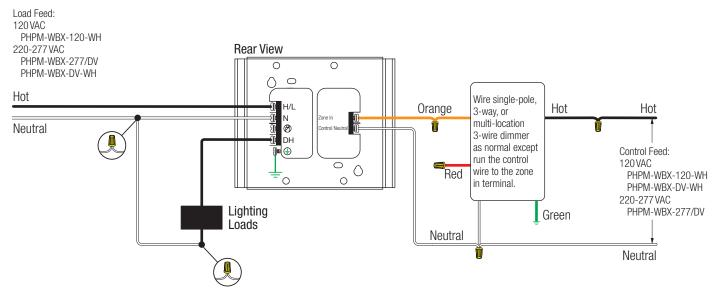
For neon/cold cathode loads select a 3-wire dimmer that has an adjustable low-end trim, since the trim may need to be adjusted. \*For Tu-Wire fluorescent loads replace PHPM-WBX-DV with a PHPM-PA-DV and wire it the same way.
