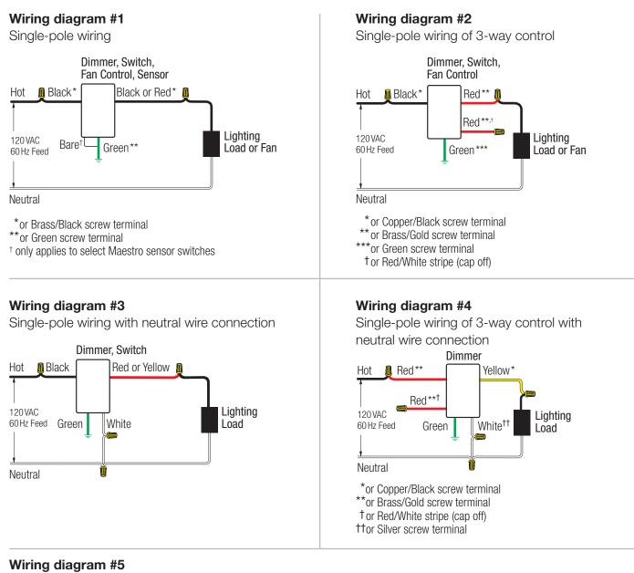
3-way wiring with neutral wire connection
