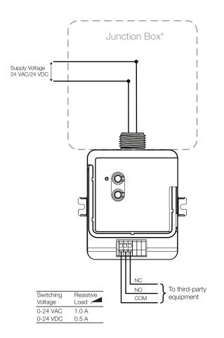
\*Some applications require the Vive PowPak module to be installed inside an additional junction box. For more information consult Lutron Application Note #423, Installing a PowPak Module inside a Junction Box, at **lutron.com/applicationnotes**.
