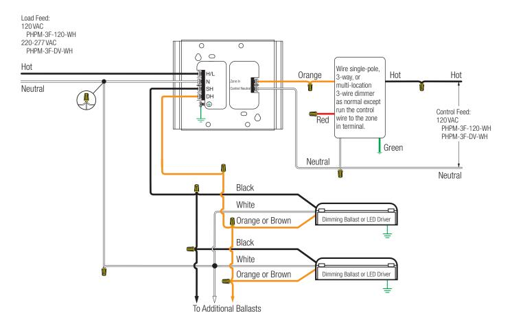
0–10V interface with 3-wire control wiring: 0–10V LED drivers, 0–10V fluorescent ballasts
