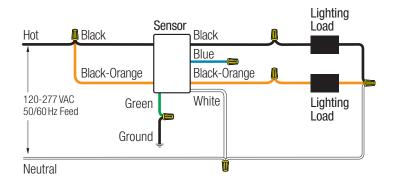
Single-pole, two breaker feed wiring for dual-circuit sensor with neutral wire connection
